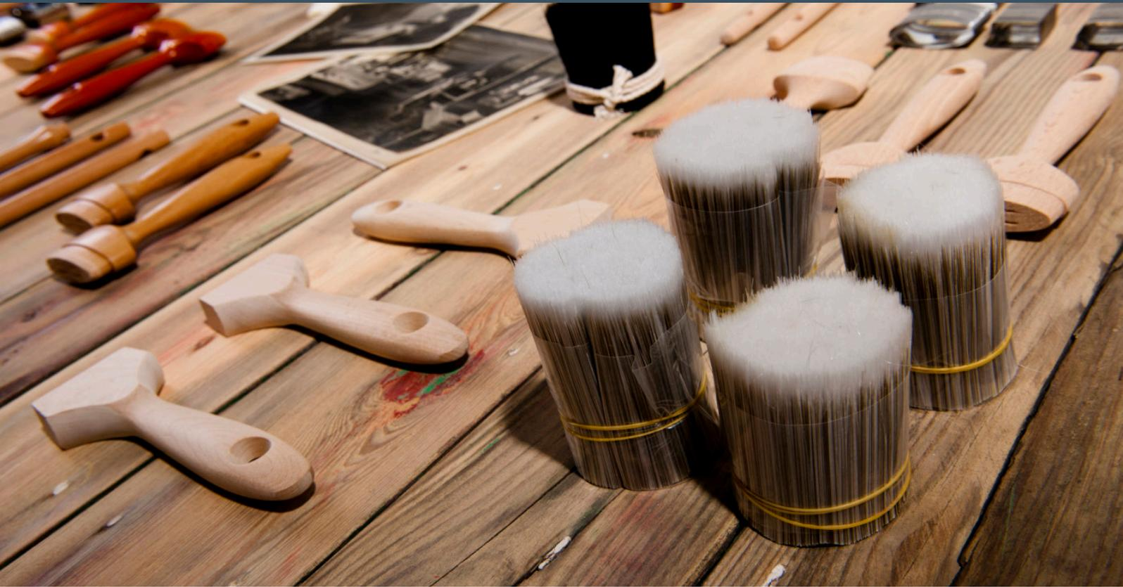
Brush heads come in many different shapes and sizes. Widths from as little as 1/2" up to 6" and in flat, oval, round and angled shapes, depending on individual preference and usage.
