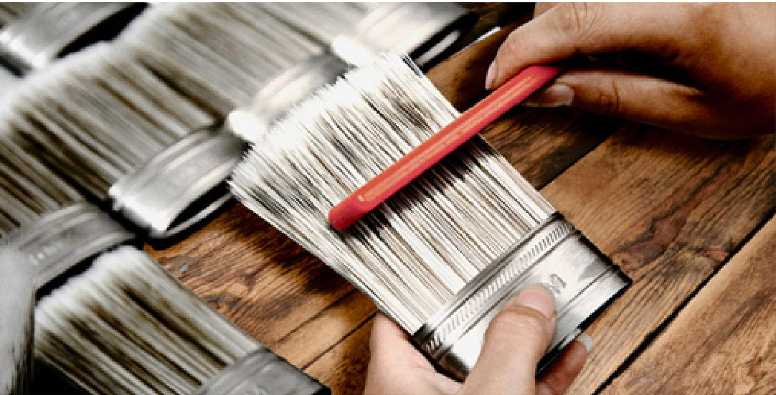
The mixture is inserted into a folded and punched seam stainless steel ferrule and tapped down so that all the filament at the base is level. This is important to ensure all the filament is locked in place during the gluing process. Wedges are then inserted to provide a paint well that acts as a reservoir to increase loading.
